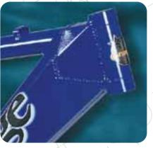
The third part of the monocoque benefit lay in how sure tracking could be by reinforcing the section joining the downtube to the headtube. By constructing the True Track head column we achieved super precise steering from a lightweight box which can have its thickness matched to the strain imposed by each individual design.
