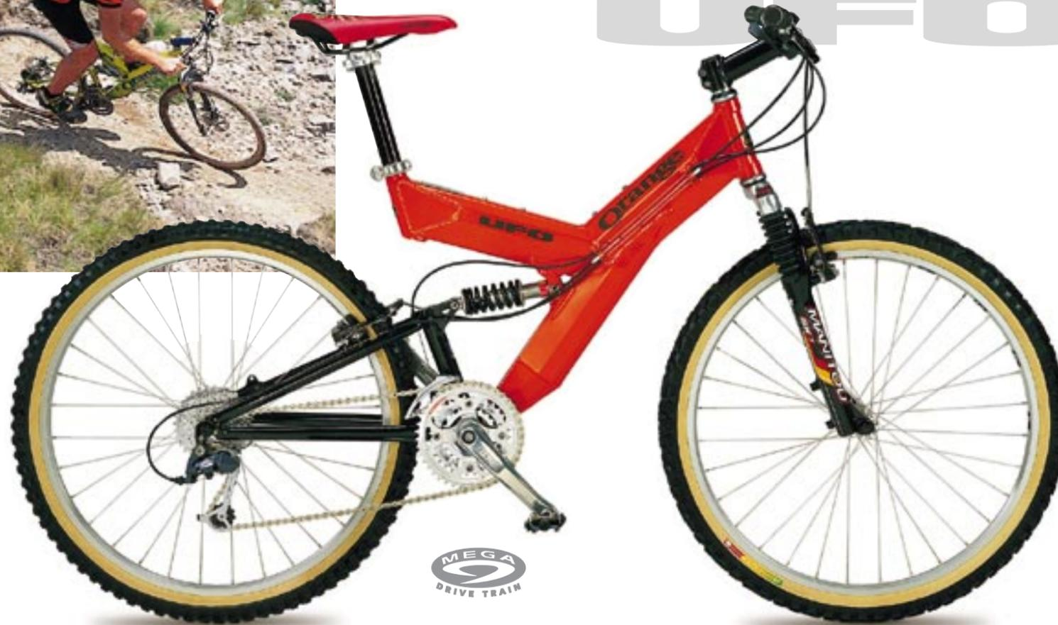
This is the first chassis to come out of the R&D department. It uses the same successful URT geometry as our X2 suspension bike, but by virtue of its monocoque front 'triangle' the UFO chassis ups the ante in the rigidity stakes. The rear triangle and shock do all the moving without having to fight against the pedal induced twisting motions of a tubular
