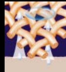
External water droplets are too large to penetrate microfibre construction.
