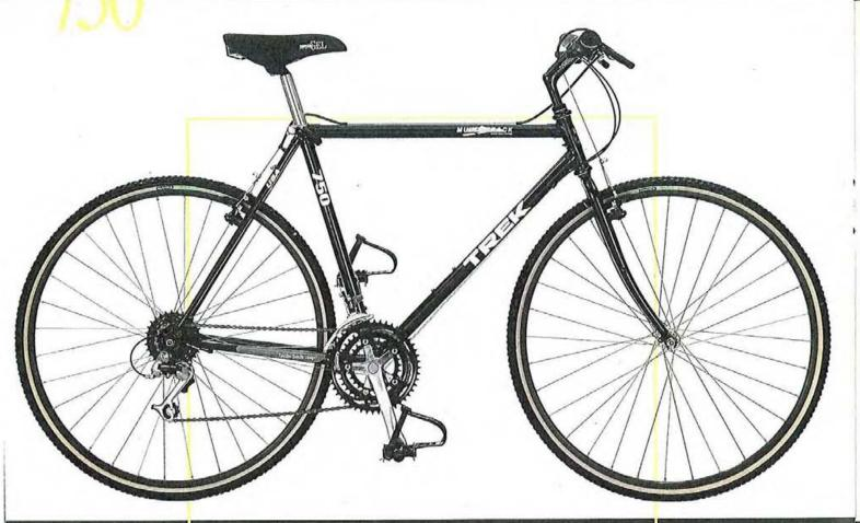
The 750 is a sport bicycle designed for comfort and fun. This double butted Cro-moly frame is driven by newly upgraded SunTour XCE components. The 750 rides smoothly with Matrix® Multi-Track tires which are mounted on durable
