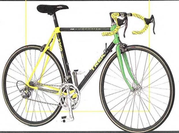
The 2100 is the latest addition to our composite line. It proves that high performance can be affordable. The 2100 features a 3 tube graphite epoxy construction which is coupled with heattreated aluminum alloy stays and fork.
