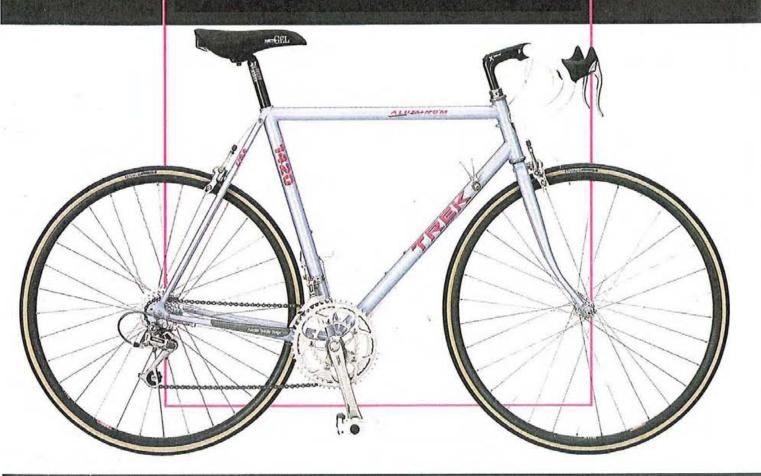
The 1200 is Trek's most popular aluminum road bicycle. It features a double butted, bonded aluminum construction which results in a strong, stiff, but very light frame. It is equipped with a Shimano RX-100 SIS drive train and Matrix® ISO-C II rims. This is a bicycle that delivers the acceleration, speed, and durability needed for riding at your best.
