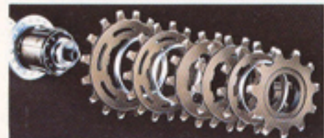
Spline-type cassette gear of Dura-Ace EX Freehub.
