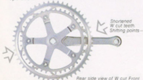
Rear side view of W cut Front Chainwheel (Dura-Ace EX)
