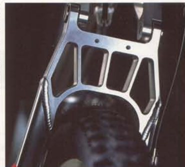
New CNC machined rear crown improves the strength and rigidity of the seatstay connection to the seat tube. Includes a removable rear brake cable stop.
