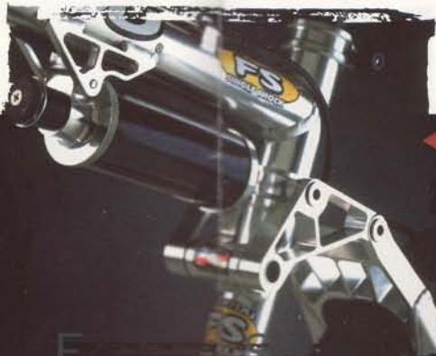
Manitou monoshock with damping controlled MCU Elastomer and Hydraulic cartridge gives 4.0" of travel.
