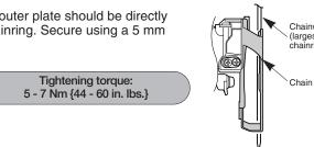
Adjust and then install the front derailleur as shown in the illustration. Do not remove the Pro-Set alignment block at this
