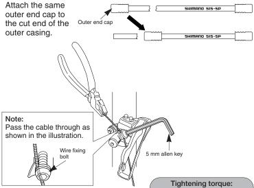
After taking up the initial slack in the cable, re-secure to the front derailleur as shown in the illustration.
