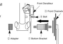
Adapter / bottom bracket tightening torque: 50 - 70 Nm {435 - 608 in. lbs.} 35 - 50 Nm {305 - 435 in. lbs.}
