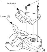
4. After checking that the indicator needle is at the right edge, install the indicator as shown in the illustration.
