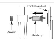
Use an 8 mm Allen key to install the front chainwheel.
