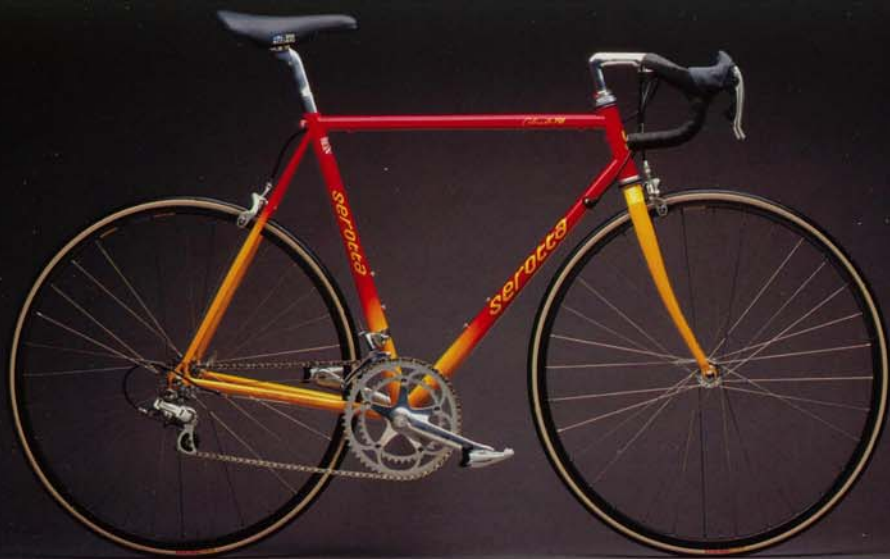
Colorado TG: Colorado Concept Steel Tubing, TIG welded, split rear brake cable guides along top tube, full braze-on fittings, semi-vertical dropouts, Serotta Power Curve chainstays, clamp-on mount for braze-on style front derailleur. Bottom bracket shell standard 68mm threaded BSC. 27.2mm seatpost. 130mm rear spacing. Prologue aluminum fork.
