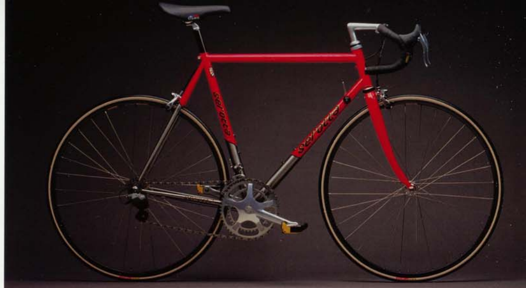
Colorado Ti: Colorado Concept Titanium Tubing, TIG welded, full braze-on fittings, split cable guides, Serotta titanium semi-vertical dropouts, Serotta S-bend chainstays, standard 68mm threaded BSC bottom bracket, clamp-on mount for braze-on style front derailleur. 27.2mm seatpost. 130mm rear spacing. Choice of composite or aluminum forks.
