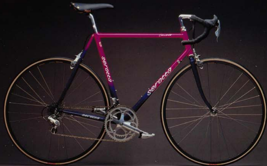
Colorado CR: Colorado Concept Steel Tubing, lugged and brazed, full braze-on fittings, side mounted internal brake cable routing, semi-vertical dropouts, Serotta S-bend chainstays. Engraved bottom bracket shell, fork crown and brake bridge. Bottom bracket shell standard 68mm threaded BSC. 27.2mm seatpost. 130mm rear spacing.
