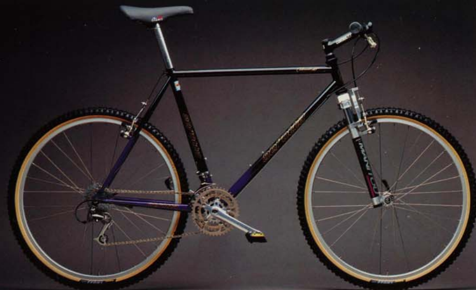
Colorado ATX: Colorado Concept Offroad Steel Tubing, TIG welded, split cable guides for brakes and gears, full braze-on fittings, semi-vertical dropouts. Bottom bracket standard 68mm threaded BSC. Headtube takes 1-inch steerer tube. 20.8mm seatpost. 135mm rear spacing. Rigid fork standard, Manitou 3 and Rock Shox Mag 21 optional.
