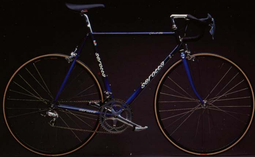
Colorado CRL: Colorado Concept Light Steel Tubing, lugged and brazed, full braze-on fittings, hand-cut lugs, side mounted internal brake cable routing, semi-vertical dropouts, Serotta S-bend chainstays. Engraved bottom bracket shell, fork crown and brake bridge. Bottom bracket shell standard 68mm threaded BSC. 27.2mm seatpost. 130mm rear spacing.
