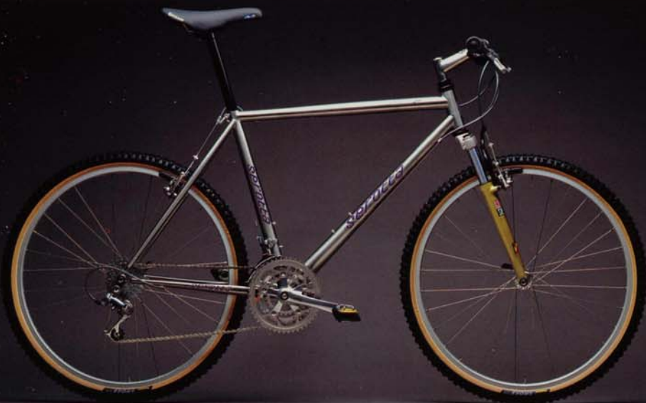
Colorado ATi: Colorado Concept Titanium Oversized Tubing, TIG welded, split cable guides for brakes and gears, full braze-on fittings, semi-vertical dropouts. Bottom bracket standard 68mm threaded BSC. Headtube takes 1 1/8-inch steerer tube. 20.8mm seatpost. 135mm rear spacing. Manitou 3 and Rock Shox Mag 21 forks optional.
