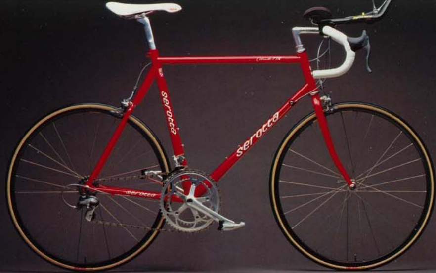
Colorado TTR: Colorado Concept Light Steel Tubing, TIG welded, split rear brake cable guides along top tube, full braze-on fittings, semi-vertical dropouts, Serotta Power Curve chainstays. Bottom bracket shell standard 68mm threaded BSC. 27.2mm seatpost. 130mm rear spacing. Prologue aluminum fork. 20-inch wheels.
