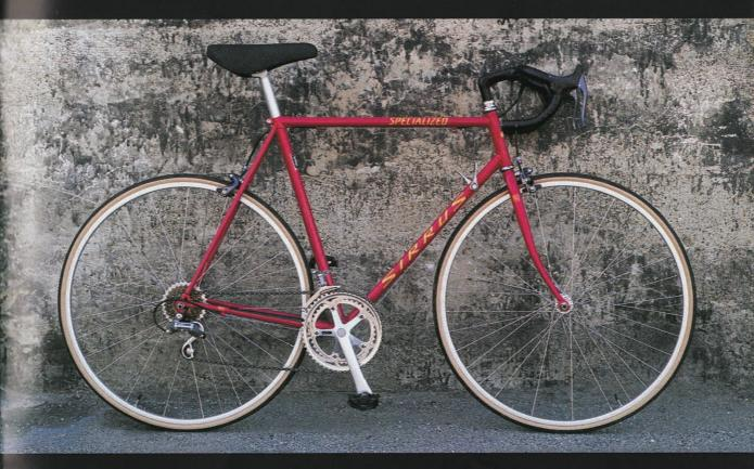
With its Specialized Direct Drive design 4130 chromoly frameset, this bike feels like a racing bike, but is always comfortable and easy to handle. The  $90^\circ$  stem allows you to use the smallest frame possible and still maintain a proper
