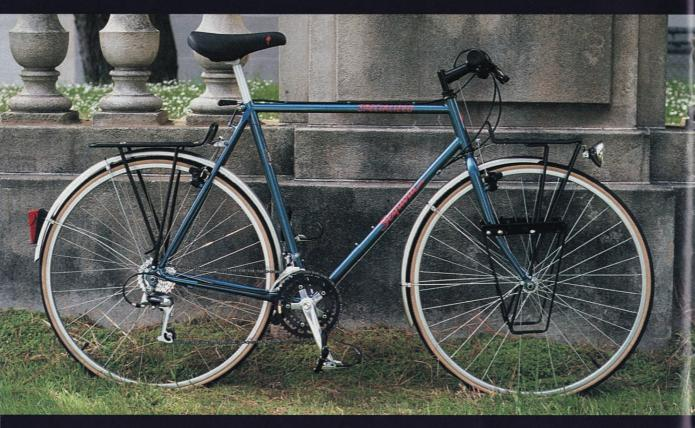
One of the best-equipped touring bikes on the market. The TIG welded chromoly frame is designed for great handling and stability. Shimano Deore LX components with upgraded Deore DX Rapid Fire shifters are positive and precise.
