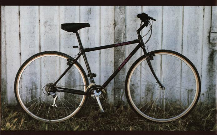
NECESSARILY, THIS CROSS BIKE HAS A FRAME THAT'S SPECIALLY DESIGNED FOR BOTH STREET AND DIRT RIDING. SUNTOUR XCT UNDER-BAR WISHBONE SHIFTERS ARE AT YOUR THUMB AND FINGERTIPS. DIA-COMPE XCT CANTILEVERS ASSURE CONFIDENT
