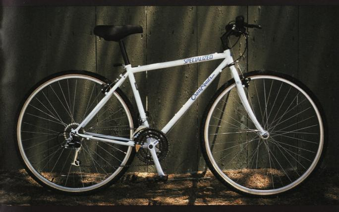
WE DESIGN OUR CROSSROADS FRAMES SPECIFICALLY FOR MULTI-SPORT USE, UTILIZING OUR SPECIALIZED FRAME SYSTEM GEOMETRY AND DIRECTDRIVE TUBING. SHIMANO 300LX GROUP WITH RAPID FIRE SHIFTERS, TO LET YOU CHANGE GEARS WITHOUT TAKING YOUR HANDS OFF THE GRIPS. ARAYA PX-45 RIMS, WHEELSMITH STAINLESS SPOKES, QUICK RELEASE HUBS AND SPECIALIZED NIMBUS 700 x 41c TIRES. 14.5, 16.5, 18, 20, 22, 18" LADIES. WHITE, BLACK.
