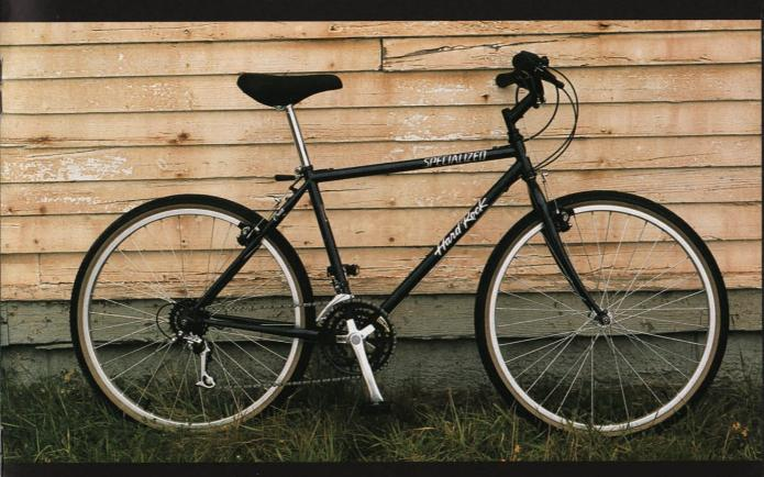
A COMFORTABLE, RELIABLE ATB. THE SFS™ CHROMOLY FRAMESET MAXIMIZES PERFORMANCE FOR ENJOYABLE, ENERGY-EFFICIENT PEDALING. SUNTOUR'S XCU ACCUSHIFT PLUS DRIVETRAIN WITH THUMB SHIFTERS ASSURES CLEAN SHIFTING OVER A RANGE OF 21
