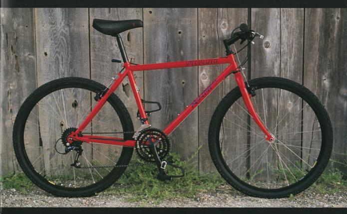
OUR SPORTY DIRECTDRIVE FRAME AND FORK, WITH CAREFULLY CHOSEN, LIGHTWEIGHT, RACE-READY COMPONENTS. THE SUNTOUR X1 GROUP WITH X-PRESS SHIFTERS GIVES YOU SURE AND QUICK SHIFTING. ROUND "POWERINGS" WITH AJS (ANTI-JAM SYSTEM) WILL
