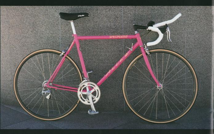
A BRUTALLY AERODYNAMIC BIKE FOR SERIOUS TRIATHLETES. THE FAST FORWARD FRAME DESIGN—78° SEAT ANGLE, 72° HEAD ANGLE—OPENS UP YOUR POSTURE FOR ENHANCED BREATHING AND A POWERFUL PEDAL STROKE. CLING-ON™ AEROBAR SYSTEM MAKES IT
