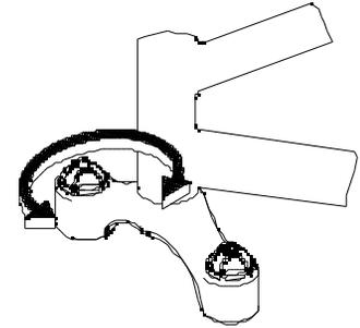
**FIGURE 16: COMPRESSION DAMPING**
