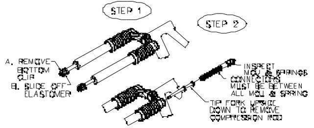
**FIGURE 10: COMPRESSION STACK**
