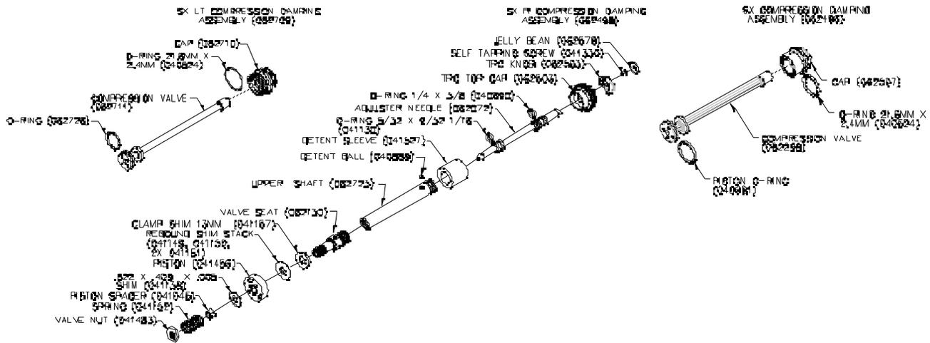
**FIGURE 12: TPC COMPRESSION DAMPING ASSEMBLY**
