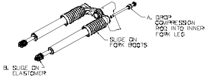
FIGURE 13: COMPRESSION ROD & BOOT
