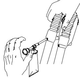
**FIGURE 7: LUBRICATING THE BUSHINGS**
