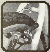
Monopoly: The Attitude uses narrow Dia-Compe 986 cantilever brakes on the rear because they stick out less than the Shimano brakes. The narrow-profile Dia-Compes avoid heel clipping. Good thinking.
