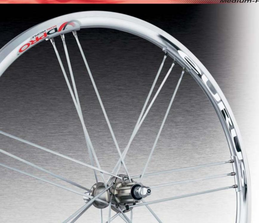
Campagnolo s's medium-profile wheels are multipurpose wheels. As light and reactive as low-profile wheels and as aerodynamic and fast as high-profile wheels. They are immediately recognizable by the unmistakable Campagnolo" G3™ spoking that sets them apart. G3™ spoking was created to provide better transmission of driving torque, better lateral stiffness and more balanced spoke tension.
