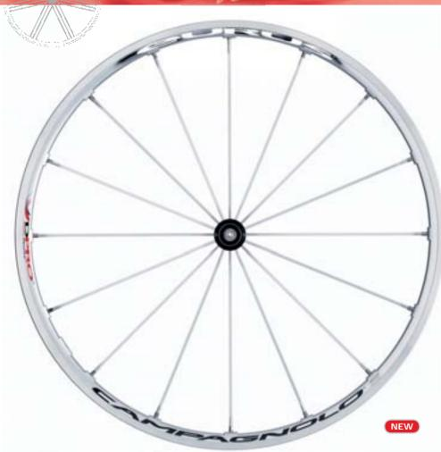
The Ultra Aero™ aluminium spokes are butted and the front wheel has radial spoking whereas the back wheel has G3™ spoking. The rear rim has asymmetrical holes to obtain a better wheel dish. The hubs are in oversize aluminium with aluminium axles and self-aligning bearings. The rear hub has a larger flange to increase torsional stiffness and therefore wheel performance during acceleration and bursts of speed on the pedals.
