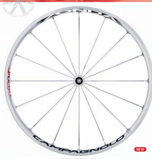
The Ultra Aero™ stainless-steel butted spokes are arranged radially on the front wheel and the rear wheel has G3™ spoking. The rear rim has asymmetrical holes to improve wheel dish.
