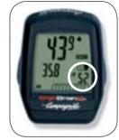
· display of chainring tooth number/sprocket in use and chain position display
