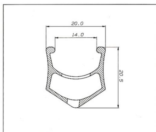
Contax has been designed for the most demanding competition. It's compact cross section design and light weight make it ideal for racing applications.
