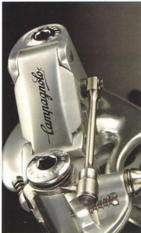
The innovative design of the CROCE D'AUNE derailleur is an improvement on the above mentioned systems and achieves its efficiency through Campagnolo's patented "TWIN-AXLE System". The "TWIN-AXLE System" is an articulation of the geometry of the derailleur which combines two movements to move the jockey cage across the freewheel while keeping it equidistant from all the cogs regardless of how big or how small they are in diameter.
