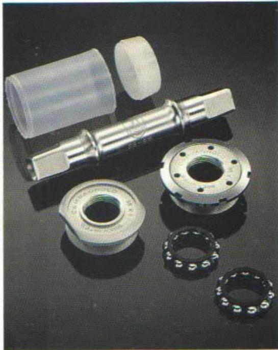
The bottom bracket is the same race-proven design that has won more races in professional competition than all others combined. It uses an axle and cups made of case-hardened steel. The rolling mechanisms are composed of hardened chromium steel balls with diameter 1/4" and held together in resin retainers.
