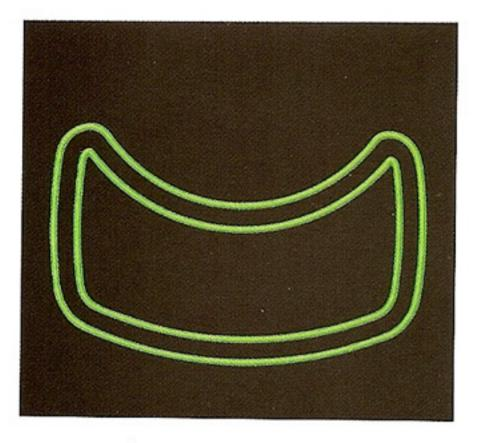
cross-sections, depending on the intended use of the rims, with the aim of obtaining the lightest possible weight, maximum transverse rigidity and optimum vertical elasticity. The cross-section was then calibrated for each rim, considering the optimum distribution of material and the mechanical effects of various geometric shapes.
