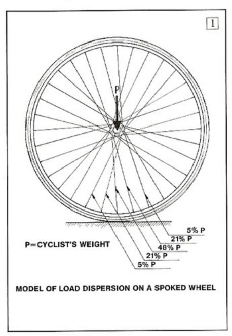
The racer's weight is applied to the hub by studying the behaviour of a spoked wheel fitted with a rim of a known profile, thickness and material, engineers have created a mathematical and physical model. This model enabled the actual stresses on the rim due to the weight to be precisely determined.
