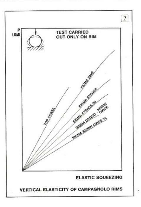
On the basis of these considerations, Campagnolo has worked out profiles and materials for its whole range of rims that solve both problems: resistance to vertical loads, and comfort for the racer.
