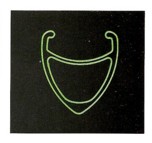
Computer design coupled with wind tunnel testing has enabled Campagnolo to design an aerodynamic rim whose profile ("V Profile") prevents the breakaway of air flow (turbulance). In comparison to a rim with a normal cross-section the special sidewall camber of this Campagnolo's rim substantially reduces the effort required to penetrate air.
