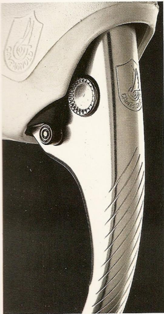
Fitting the brake lever is convenient and accessible with the use of a 5 mm. Allen bolt to attach the lever clip to the handlebar. The fixing bolt is accessible by holding the lever in the braking position. With the CHORUS brake, cables may be routed traditionally, inside the handlebar or under the handlebar tape.
