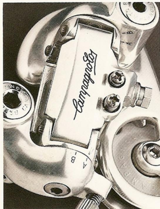
The CHORUS gear is designed in two versions, SM and LG, with different shifting capacities and biggest utilizable sprockets (see table).
