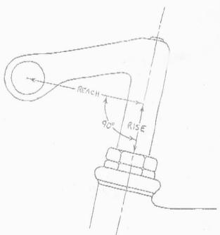
Reach specification on the 90° system is universal and can be converted to other stem angles. To convert the 90° Reach extension specified by the Conversion Chart, divide by the SIN of the desired angle and the result will be the extension in centimeters at the new angle.
