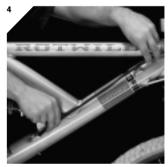
Mount the hose installation kit for the rearbrake. Measure the distance between both cablestops. Due to shrinkage, cut a length of heatshrink tube that is 10mm longer than the measured distance.
