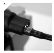
Correctly installed repaired hose on an HS 11. The barbed fitting is **flush** with the brake lever (arrow). The brake now has to be re-filled as described in the chapter 'filling and bleeding'.
