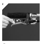
Turn the 4mm allen bolt fully counterclockwise.
