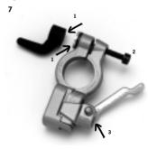
Evolution adaptor details. The black elbow can be adjusted with the toothed washers (arrows 1) as long as the fitting bolt (2) is not tightened. The elbow points preferably downwards (for better tyre clearance).
