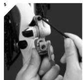
Loosen the bolts (allen key 5mm) slightly to adjust the slave cylinder. Remove the bolts if you have to switch the sides of the evolution adaptor brackets.
