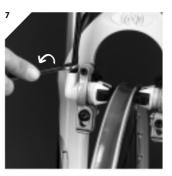
Unscrew the 8mm sleeve nut at the slave cylinder and pull out the hose carefully. Never activate the lever blade with the system open! Hold the tubing carefully in order to avoid any loss of oil!
