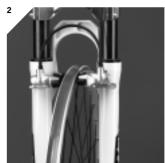
Close the quick release: Push the brake cylinder back towards the fork. Close the guick release by doing the same. That's all! A booster is not necessary with FIRM-tech and not foreseen either. It is not possible to mount one!
