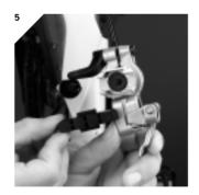
To change the brake pads; open the quick release, remove the brake from the cantistud, pull out the old pad and then just snap in a new one. After removing the wheel, pull out the old pad and snap in a new one on the other side. That's all!
