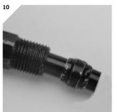
The black olive cannot be mounted incorrectly, as it is symetrical. Push the hose all the way into the slave cylinder.
