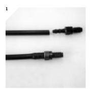
Repair of a HS 11 main hose with barbed adaptor connection.
