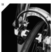
Former MAGURA models came with a silver elbow. You need a 13mm open end wrench for correct adjustment (arrow). The black and tible!
