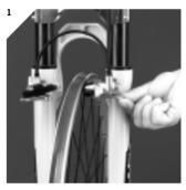
Check out the double quick release comfort! To open it push the quick release in direction of the wheel: you can now move the brake cvlinder to change your wheel or the brake
