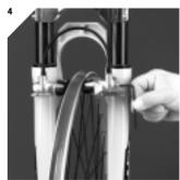
With FIRM-tech you adjust the brake pad to the rim on both sides with the 5mm allen screw. Shorten the hose and pad wear adjustment as described in the res-
