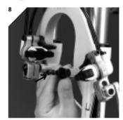
Mount a canti-stud U-washer on both canti-studs, flat side pointing up.
