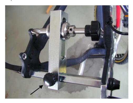
Put the quick release of the hub into the axle of the disc optimizer. Close the hand wheel of the guiding bench on the machined surface of the axle (**arrow!**). Now you can insert the axle into the dropouts of your frame or fork. Close the lever of the quick release after the faucet of the mill is positioned in the drilling.
