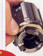
Don't over-grease as this will increase resistance in the hub, leading to chain-suck and possible derailment
