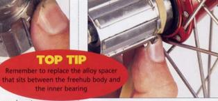
Slide the freehub body back into place. Remove the elastic band and rotate the freehub body anti-clockwise to seat the internals
