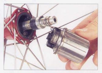
3 With the end cap removed, the freehub body should now slide off. Take care not to lose the alloy shim that sits between the freehub body and inner bearing
