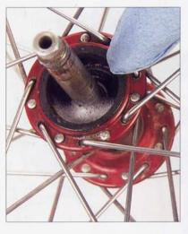
5 Degrease and wipe clean the ratchet ring in the hub body. The ratchet seal can also be removed and cleaned
