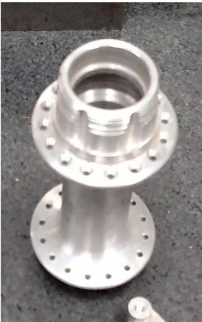
Prototype hub with the later released "wave style" rotor mount.
