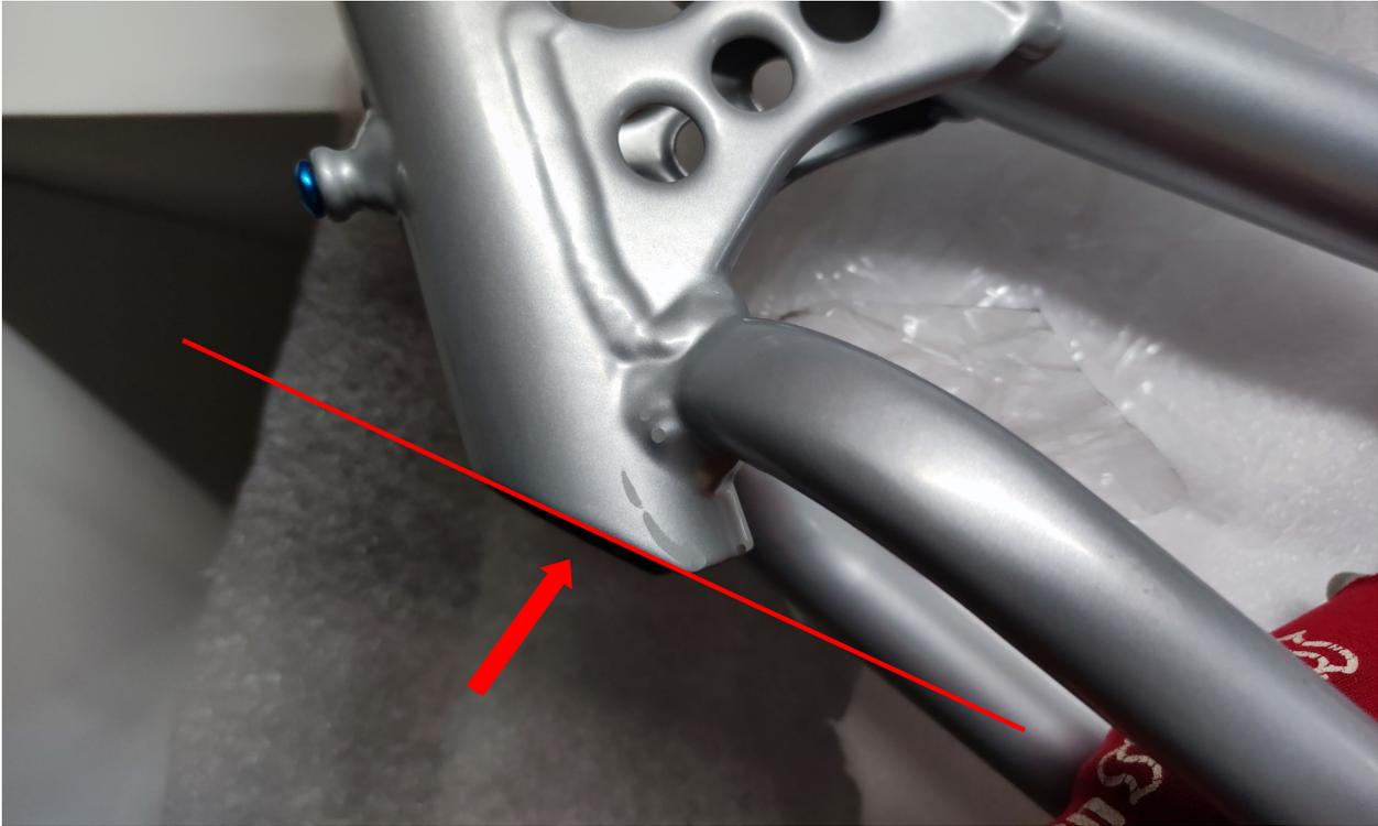
The sub frame got a cut away on the seatpost support for weight savings
