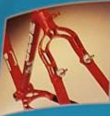
All Moho frames without rear suspension feature Mountain Cycle's exclusive Softail Traction System (patent pending), interconnected rear triangle wishbones that provide a superior shock damping effect for a smoother ride than traditional aluminum frames.
