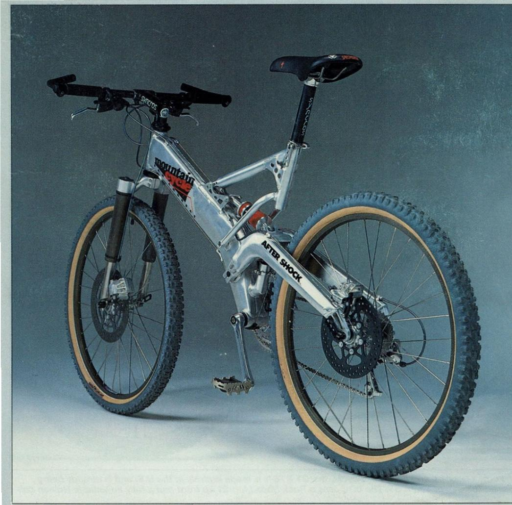
▲ **Crosstrac Sonoma:** The hydraulically suspended Crosstrac Sonoma has 4" of front and rear travel. Amazingly, the Sonoma retails for under \$2000 as a complete bike with a Shimano XT gruppo. For \$1300 you can get a frame, fork, seatpost and stem.
