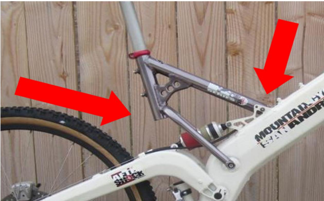
Later in the year they started to change the subframe towards the 95 model. The front clamping part lost the milled part. But the seat post tube was still cut horizontal.
