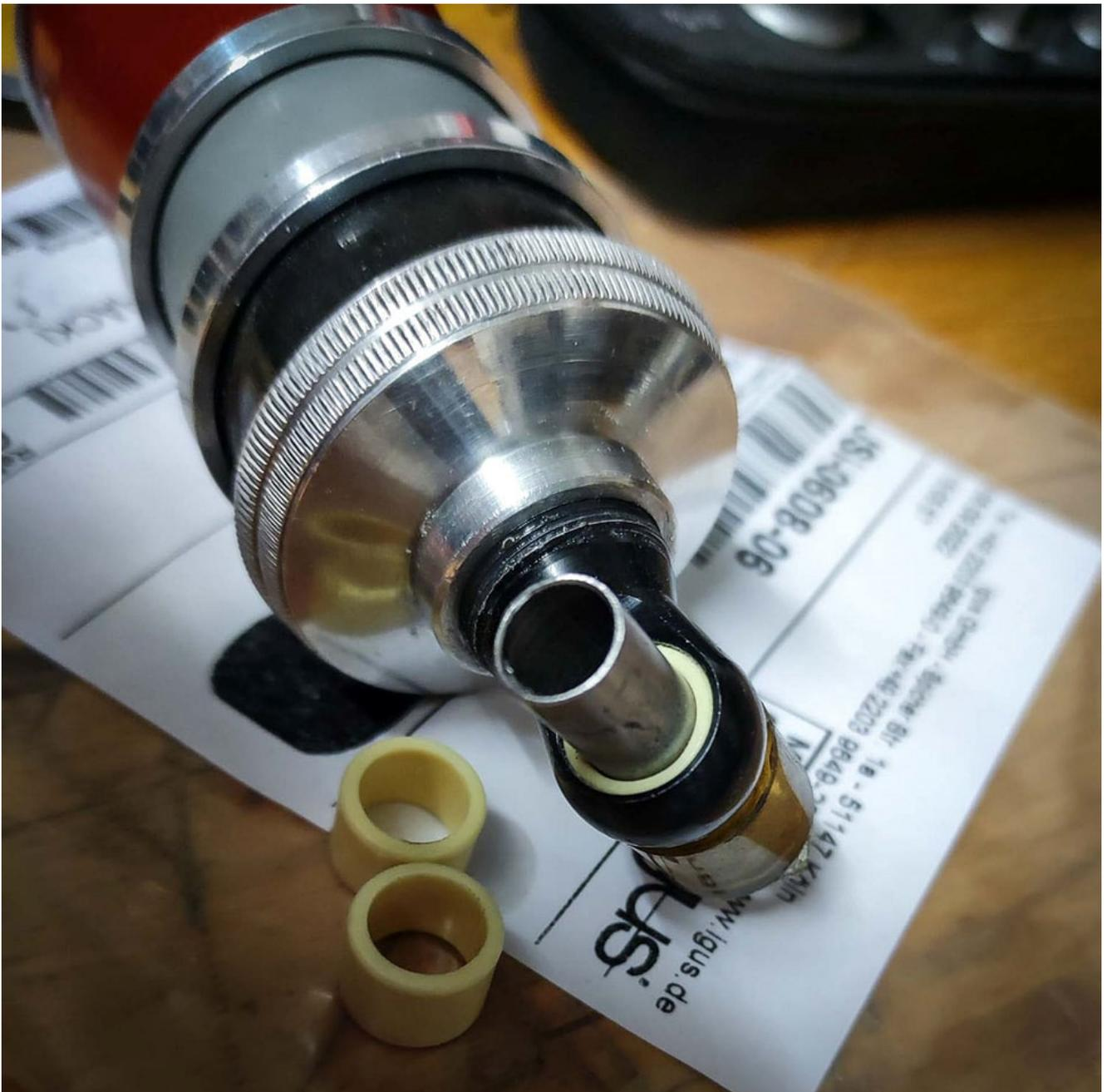
The original glide bushings are usually completely broken these days.
