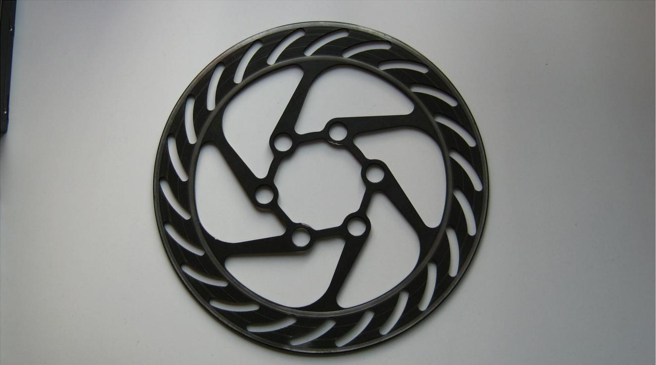
Revision of the Pro Stop discs, new with slits instead of a hole pattern
