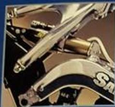
This is the heart of the San Andreas' distinctively smooth, yet responsive feel. The main frame, swingarm and subframe are all linked together at this pivotal (excuse the pun) point to yield the optimal suspension for the best ride of any monocoque suspension frame available!
