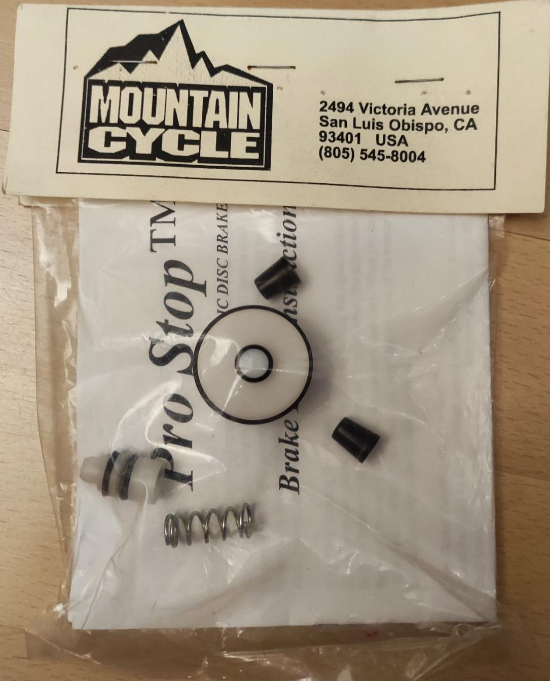
Caliper Rebuild Kit, Positive Retraction
