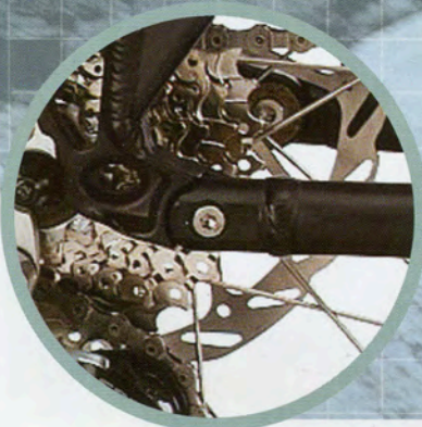
Roller bearing in all pivots for smooth, progressive long lasting performance
