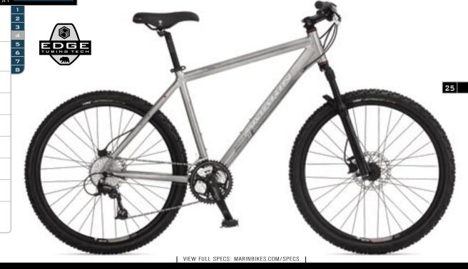
+ The Hawk Hill SE is built on a world class foundation. The frame features our custom hydroformed down tube, Triple butted 6061 tubing and disk mounts. New integrated gussets and Edge Plus II down tube provide a stiff and responsive ride.
