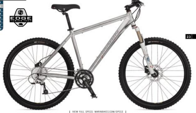
+ Careful attention is taken in order to skillfully draw double and triple butted tubes that minimize weight while increaseing strength and torsional rigidity. The Manitou Axel Super with 90-120mm of adjustment allows for custom travel tuning depending on trail conditions.
