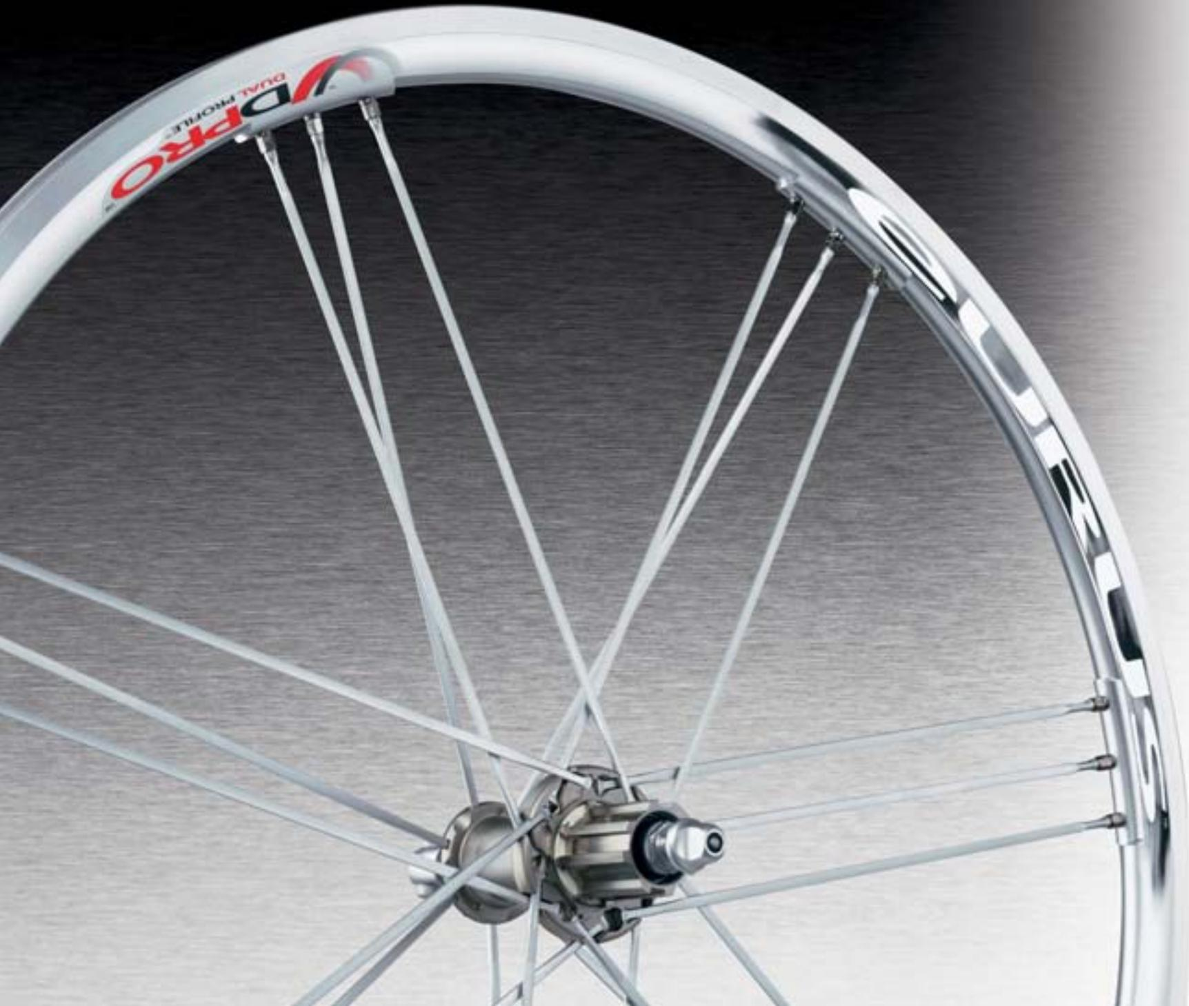
Campagnolo's medium-profile wheels are multipurpose wheels. As light and reactive as low-profile wheels and as aerodynamic and fast as high-profile wheels. They are immediately recognizable by the unmistakable Campagnolo® G3™ spoking that sets them apart. G3™ spoking was created to provide better transmission of driving torque, better lateral stiffness and more balanced spoke tension.
