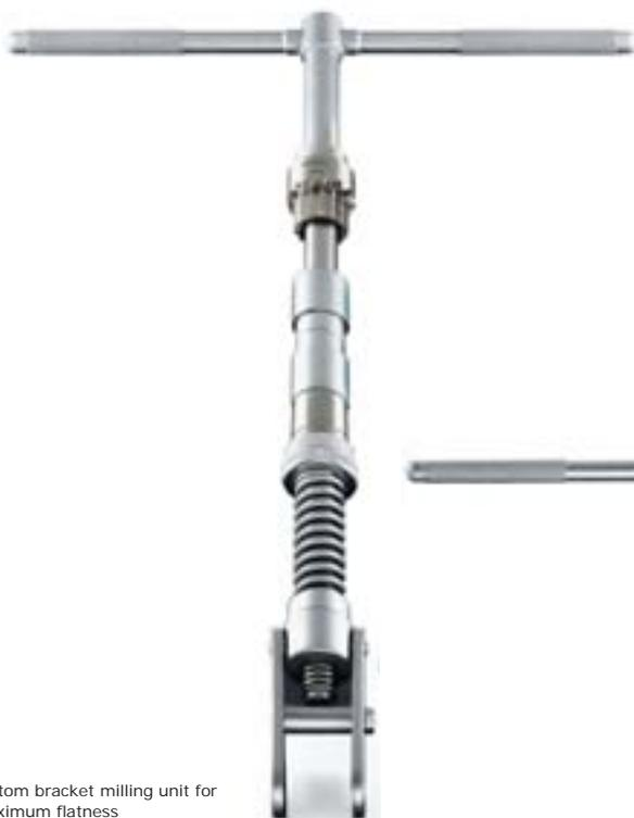
Bottom bracket milling unit for maximum flatness
