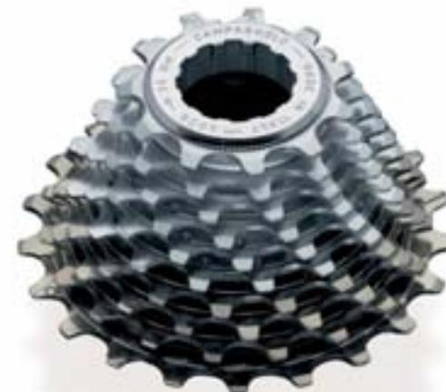
The teeth of the Record™ sprocket set have an Ultra-Drive™ design that integrates the chain and chainwheels of the crankset to ensure fast, precise and consistent shifting through the years
