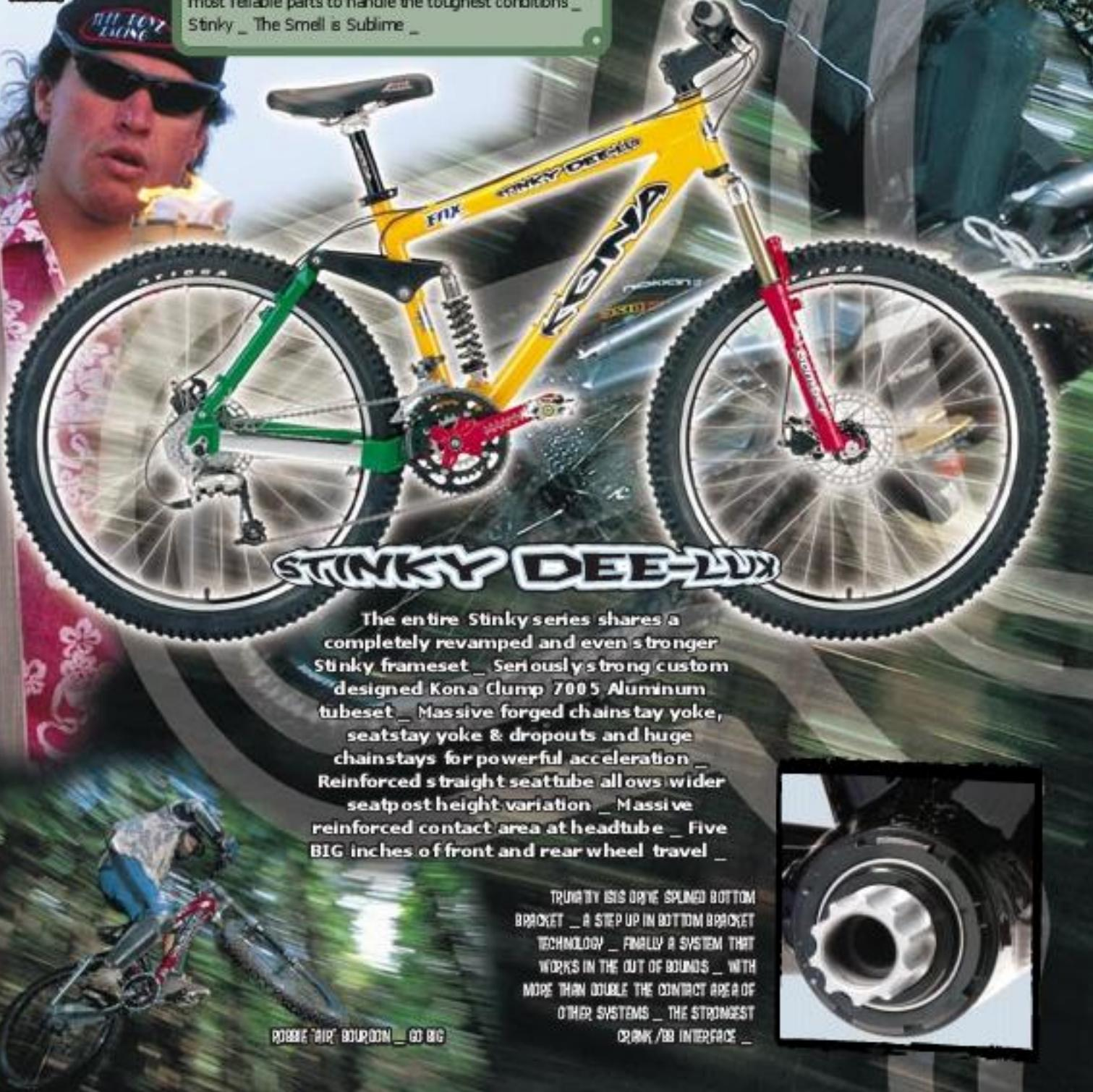
The entire Stinky series shares a completely revamped and even stronger Stinky frameset. Seriously strong custom designed Kona Clump 7005 Aluminum tubeset. Massive forged chainstay yoke, seatstay yoke & dropouts and huge chainstays for powerful acceleration. Reinforced straight seattube allows wider seatpost height variation. Massive reinforced contact area at headtube. Five BIG inches of front and rear wheel travel.
