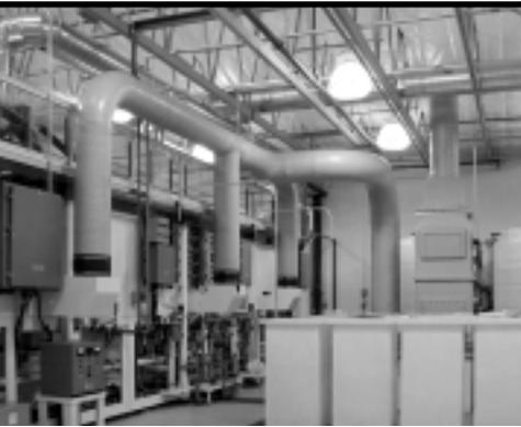
Bringing technology in-house to control and improve it is an obsession of ours and anodizing was one of the final major processes. Our new, custom designed anodizing line is fully automated, lab quality, and, best of all, recycles 100% of the water used. There is not even a drain in the floor.
