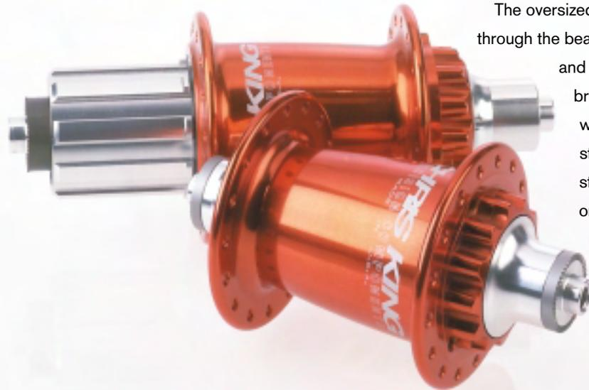
The oversized 19.5mm (completely through the bearings) axles resist the twists and flex associated with disc brakes and suspension frames while high flanges build strong wheels. For added strength and stiffness, a bolt-on axle is available (rear only). Originally designed for cross country use, our hubs are also some of the lightest available (150g front; 282g rear).
