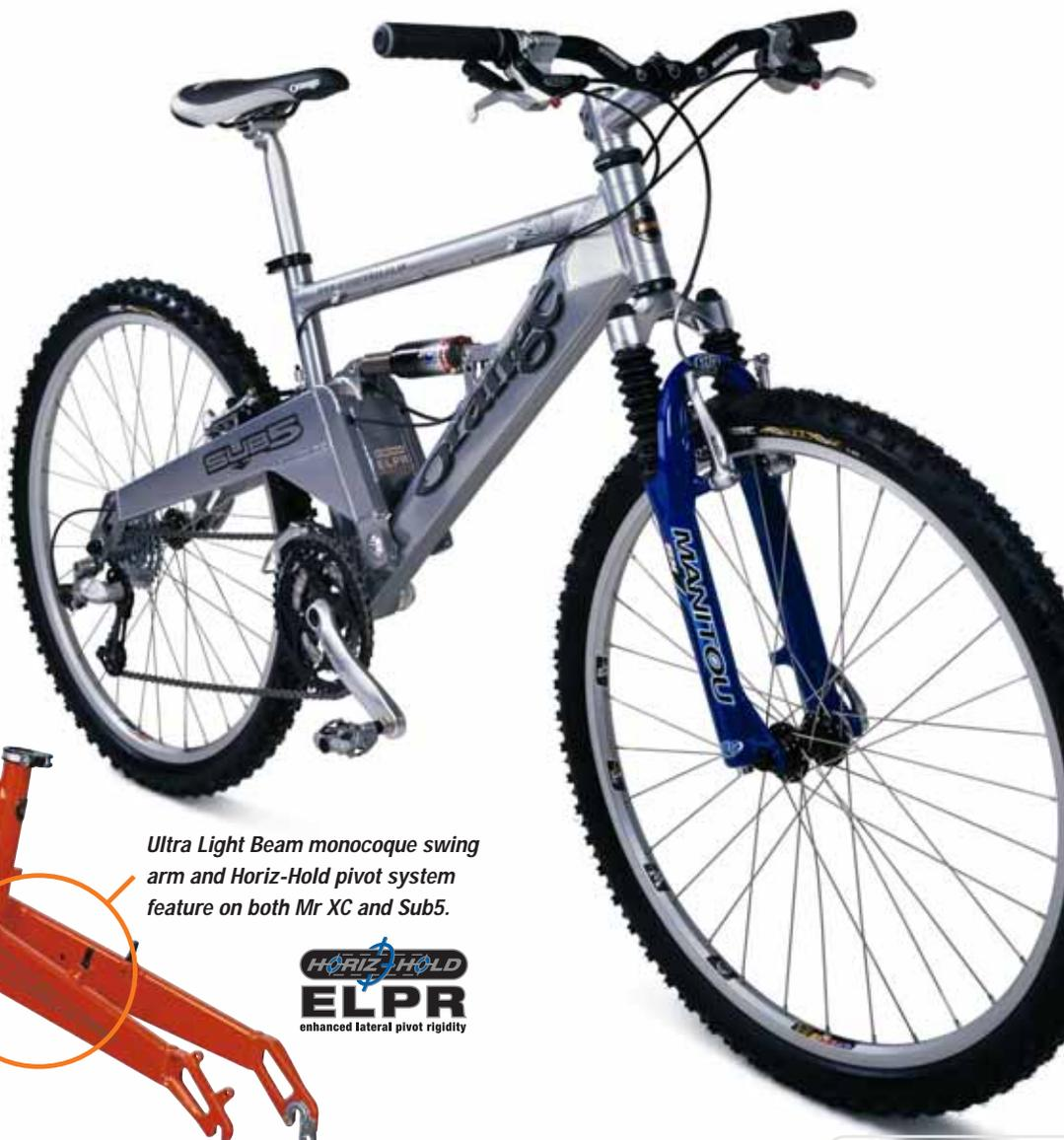
**Ultra Light Beam monocoque swing arm and Horiz-Hold pivot system feature on both Mr XC and Sub5.**
