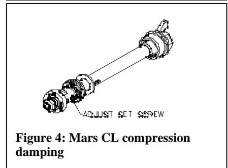
**Figure 4: Mars CL compression damping**
