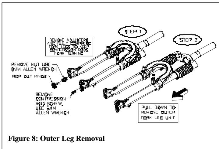
**Figure 8: Outer Leg Removal**
