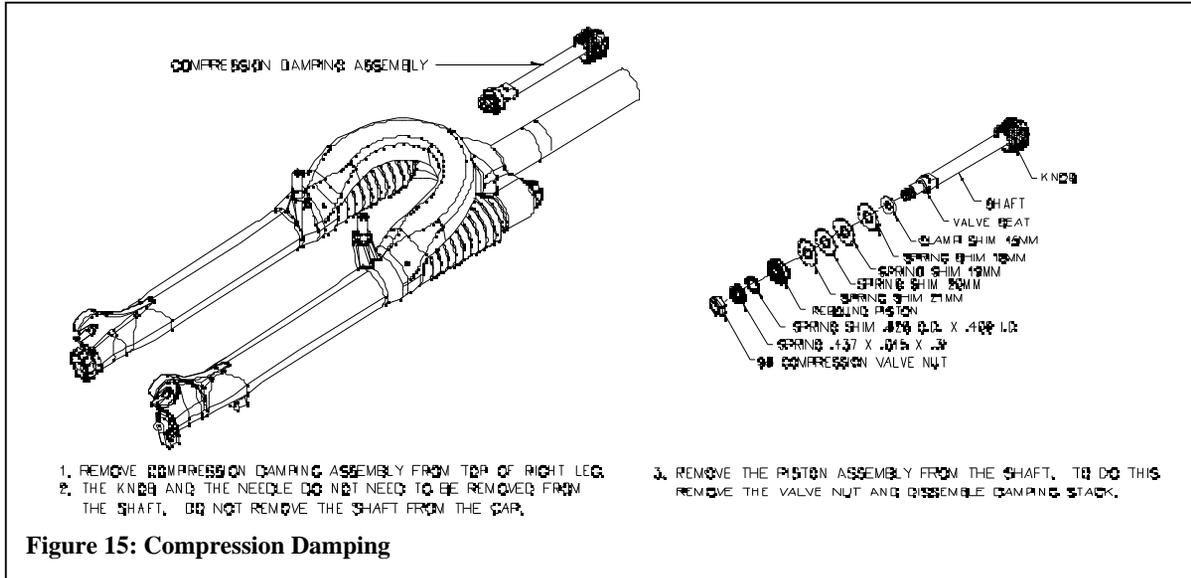
Figure 15: Compression Damping
