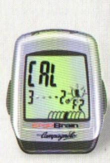
The first and only integrated computer to indicate not only the position of the chain but also the number of teeth for the chainring and sprocket in use.
