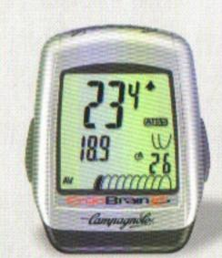
The retro-illumination switches on when a function is activated. As soon as the buttons are touched, it remains on long enough to read the display or select a new screen. When the computer returns to stand-by, at the end of the training session, the function is automatically disabled to avoid accidental use during daytime rides.
