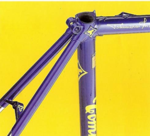
Cadre "11 tubes" Columbus E.L. oversize (acier Nivacrom). Pièces microfusion exclusives
