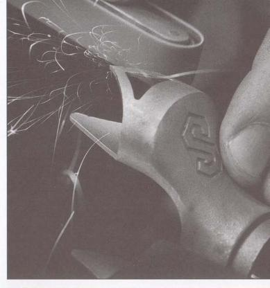
Preparation of a Classic steel fork. In traditional lugged / brazed frames all parts are cast to tightly controlled Serotta specifications. All contours are painstakingly prepared for aesthetic appeal and sockets are checked for proper fit-up. For durability, all stress rising burrs are removed. It's in time consuming details like these that Serotta's break away from the peleton.
