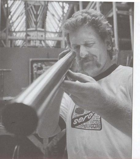
**Spec's aren't everything...** Don Chandler's knowing eye checks each tube for surface blemishes which are not necessarily picked up by instruments.
