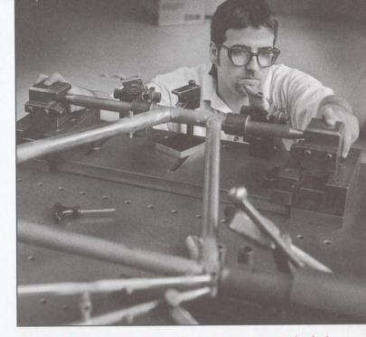
Throughout the assembly process frame components are checked for alignment. Unlike most companies who will check alignment only at the end of production, Serotta makes repeated alignment checks to eliminate the potential for significant alignment adjustments which can take "life" out of new frame materials. Here, John Otoupal makes the "final" alignment inspection on a new Atlanta frame.
