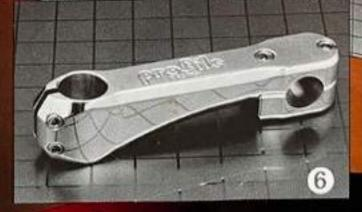
Engineered for extra strength demanded by downhill and dual slalom racing- CNC machined from 7075-T6 billet aluminum- Threadless clamp-on style for 1" and 1.125" steezer tubes-Zero degree rise-Available with 105mm, 120mm, or 135mm extensions-Supplied with aluminum spacers and top cap. Available in polished and color finishes.
