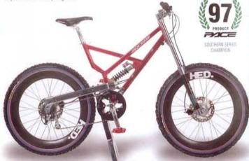
Other standard features include load dedicated external frame butting, service free bearings, disc-brake ready design, detachable seat sub-frame (available in three position configurations), fork lock-stop, detachable drop-outs and oversized butted headtube.
