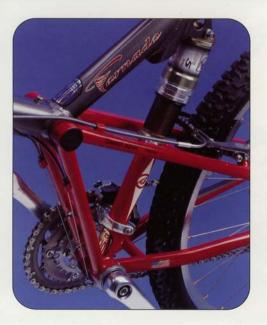
The Breezer Tornado and Twister both feature Joe Breeze's adaptation of the Sweet Spot Unified Rear Triangle design. This suspension has earned widespread acclaim for its plush ride, superior traction on all terrain, generous travel, and resistance to pedalinduced actuation (the dreaded "bob").
