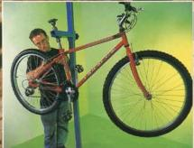
Saracen's polyester powder coat is electrostatically applied over a chromate rust proofing primer, and baked at 180°C. Its then carefully inspected to make sure every bike starts with an immaculate finish
