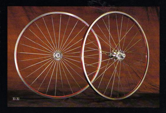
are about half the weight of stainless. Because the Ti blades are stronger and harder to break than stainless, we can use fewer spokes. Fewer spokes also means lower wind resistance. If you make a comparison to a 32 spoke three cross wheel that uses 14-15 gauge butted spokes the weight savings is 92 grams for the spokes alone (over 3 1/4 ounces per wheel). This is weight reduction where it counts and it produces a difference that you can feel.
