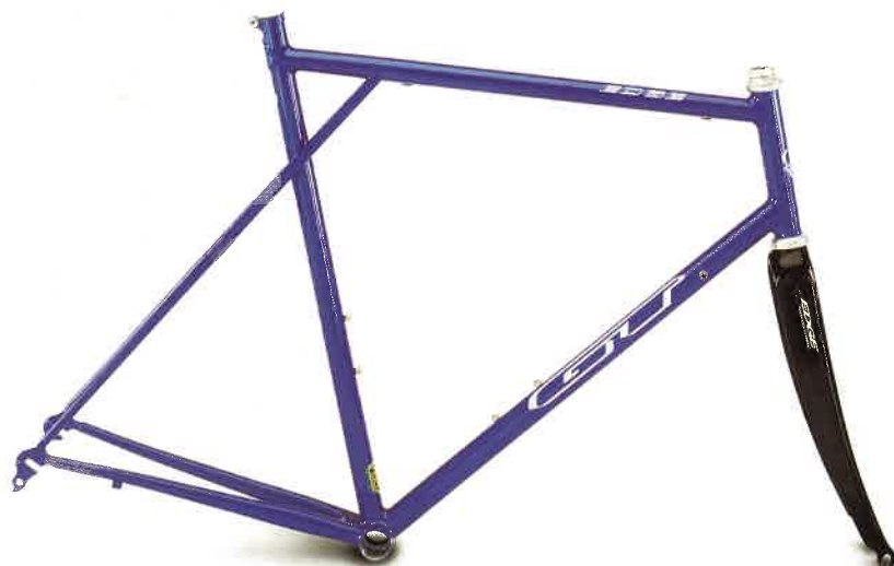
FRAME: GT Road design Reynolds™ 853 butted Cr-Mo tubing, made in the USA FORK: Edge carbon fiber aero blades SEAT POST CLAMP: Braze-On COLOR: Blue, Red, Black, Pearl White, Yellow, or custom per order SIZES: 48, 50, 52, 54, 56, 58, 60cm Headset not included
