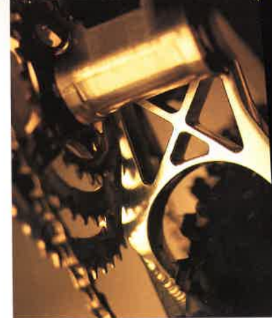
In cross-country competition (top left) or downhill, Team GT put the STS through the most rigorous testing possible. Above: the CNC-machined X-brace lower pivot of the STS.
