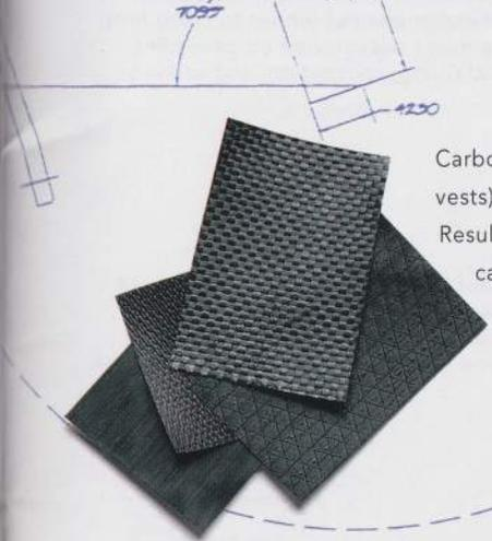
Carbon and Twaron (the stuff of bulletproof vests) are custom-layed up in huge molds. Result: extraordinarily lightweight and strong carbon fiber frames.
