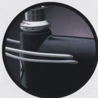
**1** Integrated, internal brake cables attached to Magura Race Line brakes, some of the surest stoppers in the brake business, inspiring confidence at every turn in the trail.
