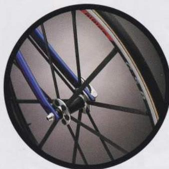
**3** Very hot wheels: replaceable carbon fiber aero spokes designed by Giant's carbon whiz, Mike Burrows, combined with Rigida DP aero rims, mean extreme strength and blazing aerodynamics.
