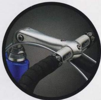
**1** The key to Compact Road Geometry is this Mike Burrows-designed adjustable stem. It lets you dial in the fit and feel you want, while riding no more frame than necessary.
