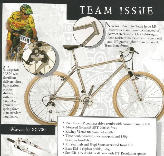
Marzocchi XC-700. The ultimate suspension system. 1380 grams, 51mm travel. 6-position externally adjustable speed sensitive valving. New dust wiper with integrated weather boot for improved reliability.
