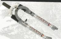
Marzocchi Zokes suspension fork. 1440 grams. 51 mm travel. 6-stack Elastomer with allen key pre-load adjusters.
