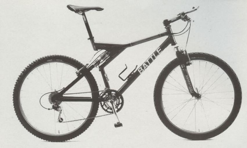
long section of seat tube above the bottom bracket accommodates a host of derailleur and chainring options. Welding and construction on the 6061 T-6 frame is superb. All pivots ride on permanently lubricated composite bushings, including the robust Horst Link dropouts.
