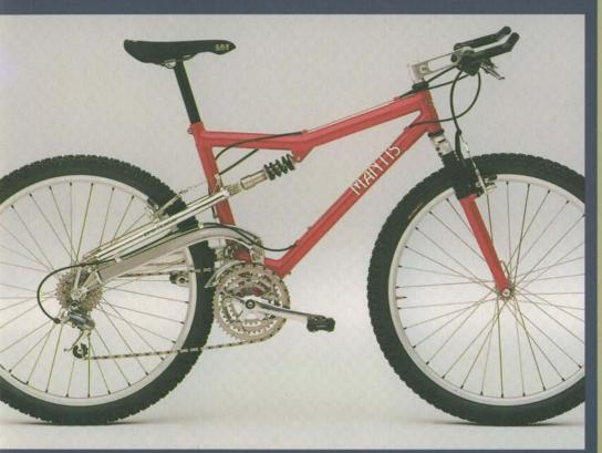
The Pro Floater is one of the original, all time great full suspension bicycle frames. It is a McPherson strut bike, because the McPherson strut design is fully active, resists flex more efficiently, and is simpler to use than any other type of rear suspension. The triangulation of the swingarm and compression strut holds the rear wheel in place with less material than any other type of rear suspension.
