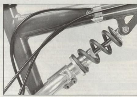
Titanium at work: The Dagger came with a choice of a Risse air shock or an AMP thru-shaft damper. Surprisingly, both shocks suffered AMPphysema—the hissing noise that occurs on the rebound stroke. Most of the test riders preferred the AMP shock for its longer travel and lightweight titanium spring.
