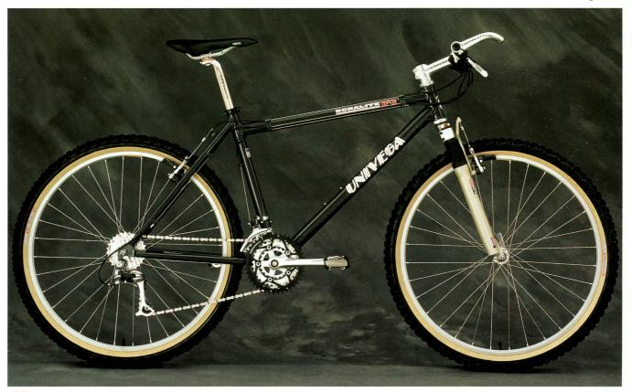
Tunivega suspension specific MTB w/TIG-welded B4C advanced metal matrix composite tubing, sloping T/T and forged dropouts. Sold as frame only.
