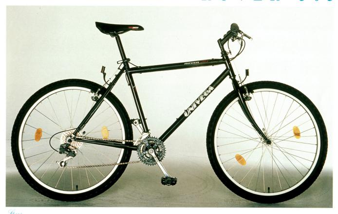
Frame 26" Univega MTB design w/Formula chromoly tubing and sloping T/T. Fish 26" MTB unicrown; high-tensile steel w/safety dropouts. The proposition of the propositi
