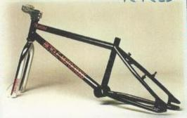
This is the number one BMX frame in the world today. A classic design with revolutionary technology. Tange Prestige and Reynolds 531 double butted tubing, chrodropouts, 21" top tube length, tapered chainstays from 7/8" to 3/4", flared 1" seat tube, and
