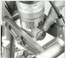
Hidden pleasures: The extra beef in the FSR's linkage is a testament to Specialized's designed-in reliability. Tucked between the FSR's moving parts is the Fox ALPS rebound adjustment knob. The entire bike had a purposeful look to it.
