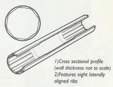
This brand new racing tube set introduced in 1992 features doubled butted, oversized main frame tubes, with laterally aligned stiffening ribs on the butt sections to maximise stiffness and tortional rigidity, as with the 708 Classic set. 731 OS race is approximately 10 % lighter than comparable competitive tube sets, and is suitable for road, track and time trial frames at professional level.
