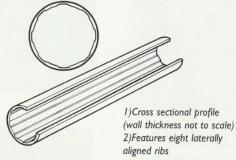
A recent development from Reynolds, the name describes the purpose. The main tubes of this set have a new and ingenious internal profile. The profile is designed to maximise lateral stiffness and strength in the directions of the known loadings, which result from the punishing road surfaces and the extreme rider applied deflection loadings experienced on the brutal classic racing courses.
