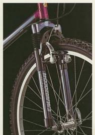
strength to weight ratio, titanium top and down tubes combine with a hand brazed cromo rear triangle to improve traction and climb, whilst providing truly responsive power transfer. Highly specified with Shimano groupsets, titanium bars, light cromo forks and with Pace RC35 Kevlar suspension fork and
