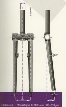
Based on the geometry of our successful Team Raleigh bikes, the angles and rakes have been refined to provide a comfortable yet resilient and responsive ride. Special features include external alloy cable guides and hand forged vertical drop outs.
