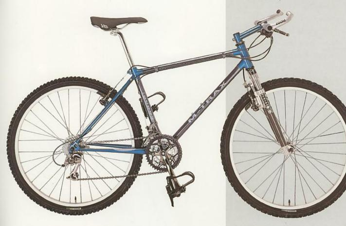
The model shown is the Ti2000s, fitted with the optional PACE Kevlar/carbon suspension fork.
