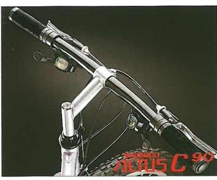
A step over design frame built using Reynolds CR-MO tubing and equipped with Shimano's simple to use C90 18 speed S.T.I groupset ensures comfort and convenience when using the Sajitta.
