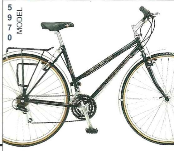
A versatile bicycle designed for simplicity and smooth function. SRAM Gripshift gives excellent control of the Shimano gears. A sensible selection of accessories complete the Legend.
