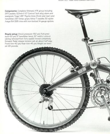
Frame dimensions: Seat tube length (center to top)-18"; Top tube length-22"; Chainstay length-16.9"; Bottom bracket height-11.625"; Wheelbase-41.5"; Head angle-71"; Seat angle-73.5"; Actual frame size-17.5".
