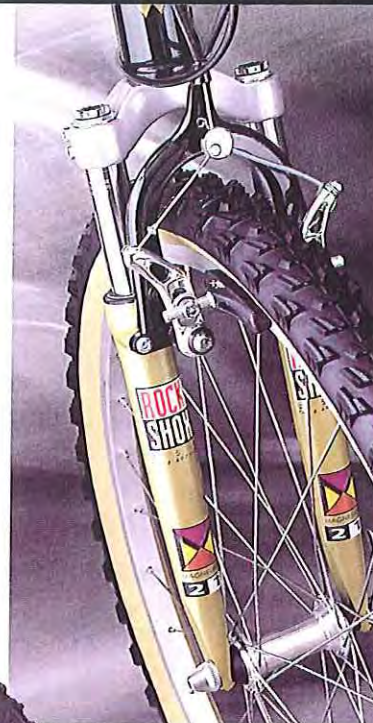
Serious Spec: Rock Shox Mag 21 air/oil suspension fork. Ultimate responsiveness on all types of terrain.
