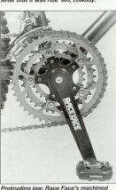
Protruding jaw: Race Face's machined aluminum I-beam crankset was superstiff. Unfortunately, the Syncros titanium bottom bracket pushed the crank far to the right and out of sync with the drivetrain.
